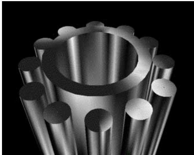
Simplified diagram of Searl's system of magnetic rings and rotating magnetic rods.
